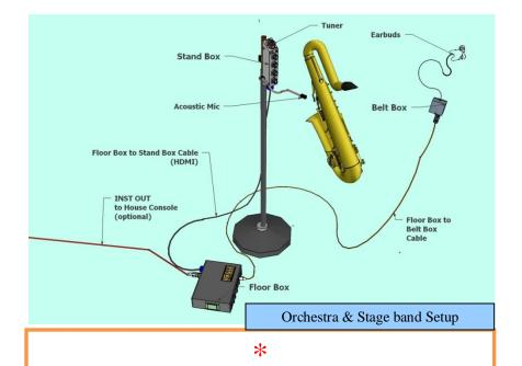
In the example shown above, POSSE is being used for monitoring of the instrument only. A Singer/instrumentalist could use the vocal mic as well. If the House mixer chooses to, the Instrument Mic signal can be added to the House mix via the INST OUT jack on the Floor Box.
