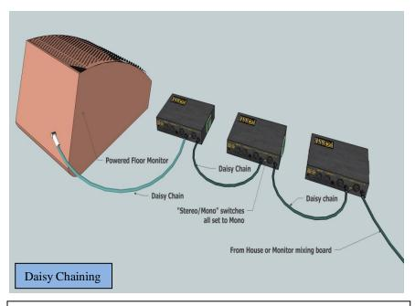
Several POSSEs and powered stage monitors (in any order) can share a common monitor mix. In the example above, the monitor mix is being sent to the AUX IN R on the 1<sup>st</sup> POSSE (far right) and then daisy chained to the others, via AUX IN L. AUX inputs must be switched to MONO.
